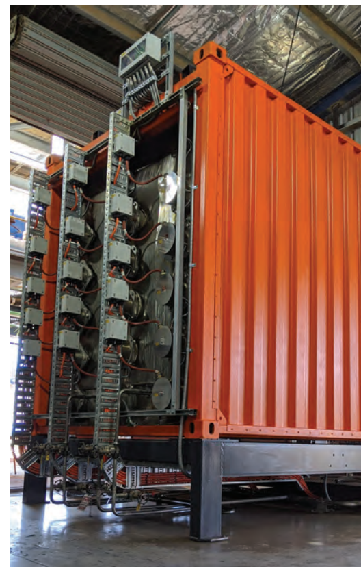
1MWh thermal energy storage unit constructed by Graphite Energy
