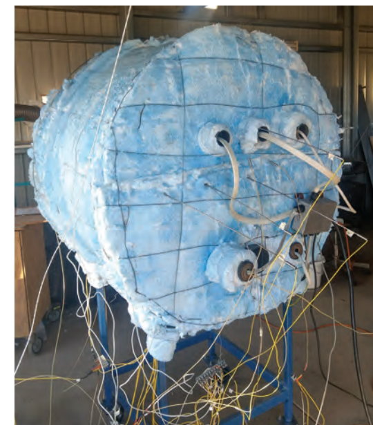
Electrically charged PCM hybrid for production of heated air (up to 700°C) successfully tested at UniSA
