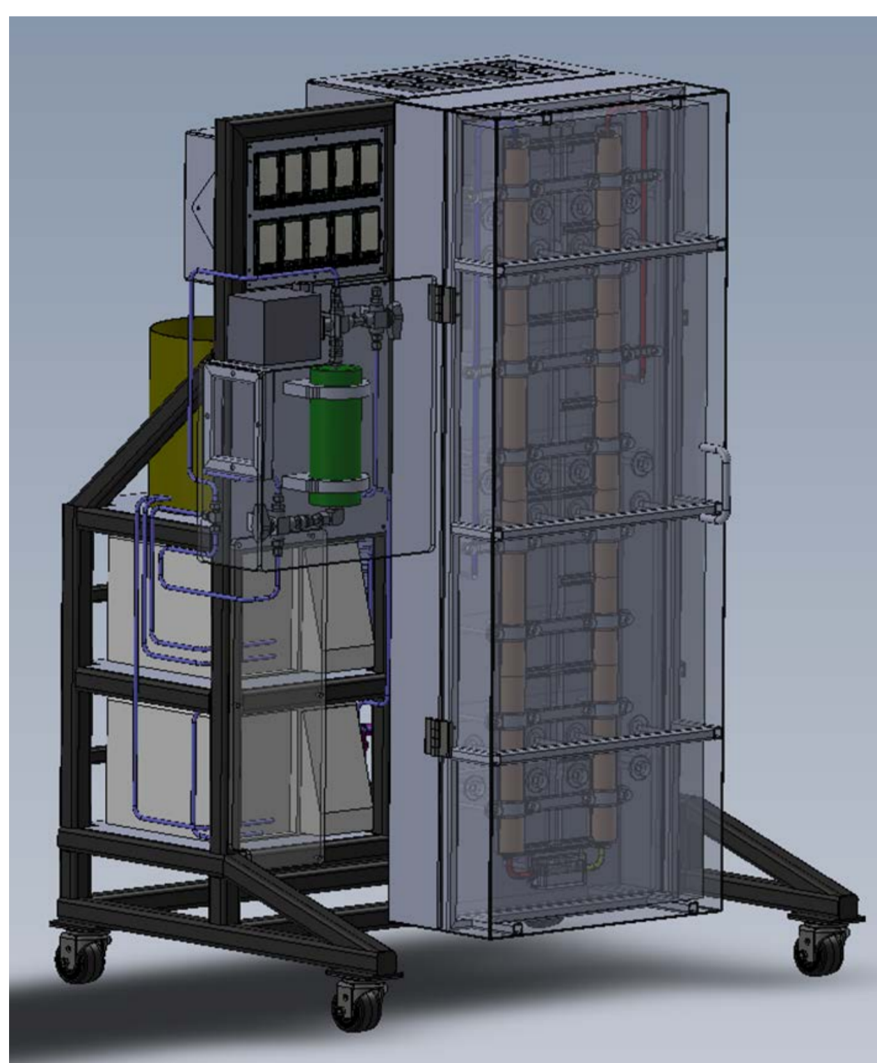
Figure 2: Lab scale continuous-flow tubular apparatus for supercritical water gasification of algae
