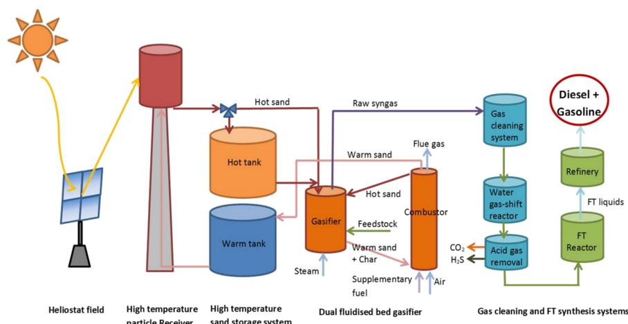
Figure 1: Schematic diagram of solar-to-liquids system via SDFB gasifier.
