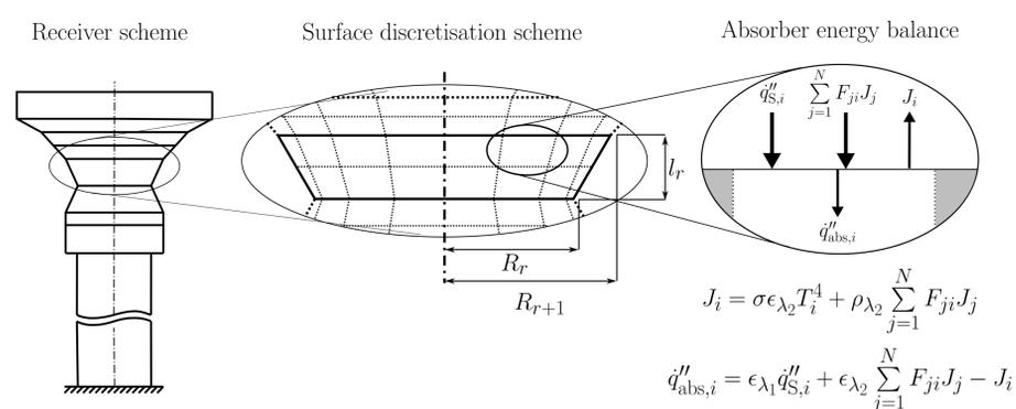
Figure 2: Tower receiver geometry class example with variable geometry parameters and wall energy balance scheme.
