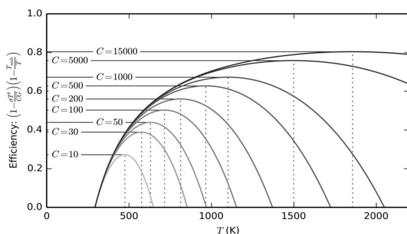
Figure 1: Efficiency of conversion of radiation into work as a function of temperature for a series of optical concentrations
