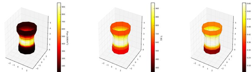
Figure 3: Sample flux, temperature and efficiency distributions for a candidate of a simple class of FONaR geometries.
