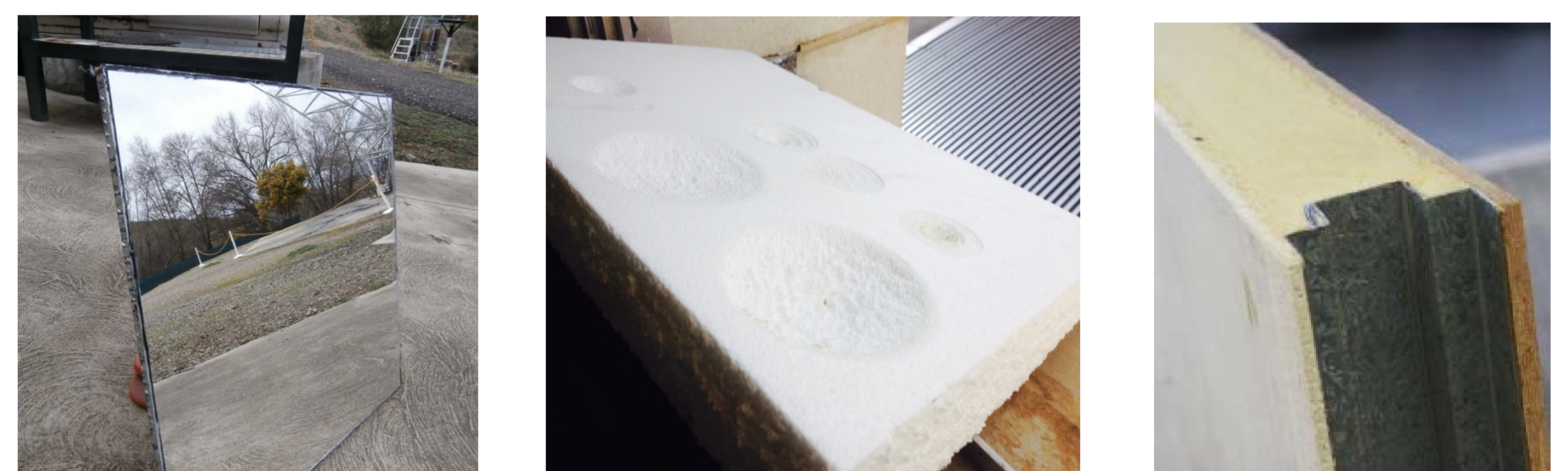
Figure 4: Prototype aluminium honeycomb mirror (left), trials of laser cut EPS (centre), and PU-cored structural wall panels used as a basis for new mirror panel designs (source: APC Manufacturing and Logistics Pty Ltd).
