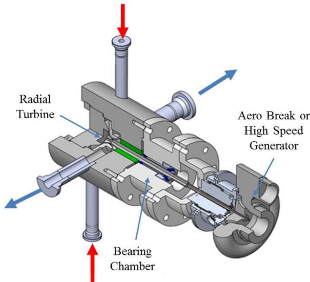
Figure 4.21: First iteration of a concept for small scale sCO<sub>2</sub> turbine, developed in 2016
