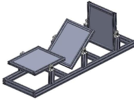
**Figure 4.31. Solar mirror test-rig**
