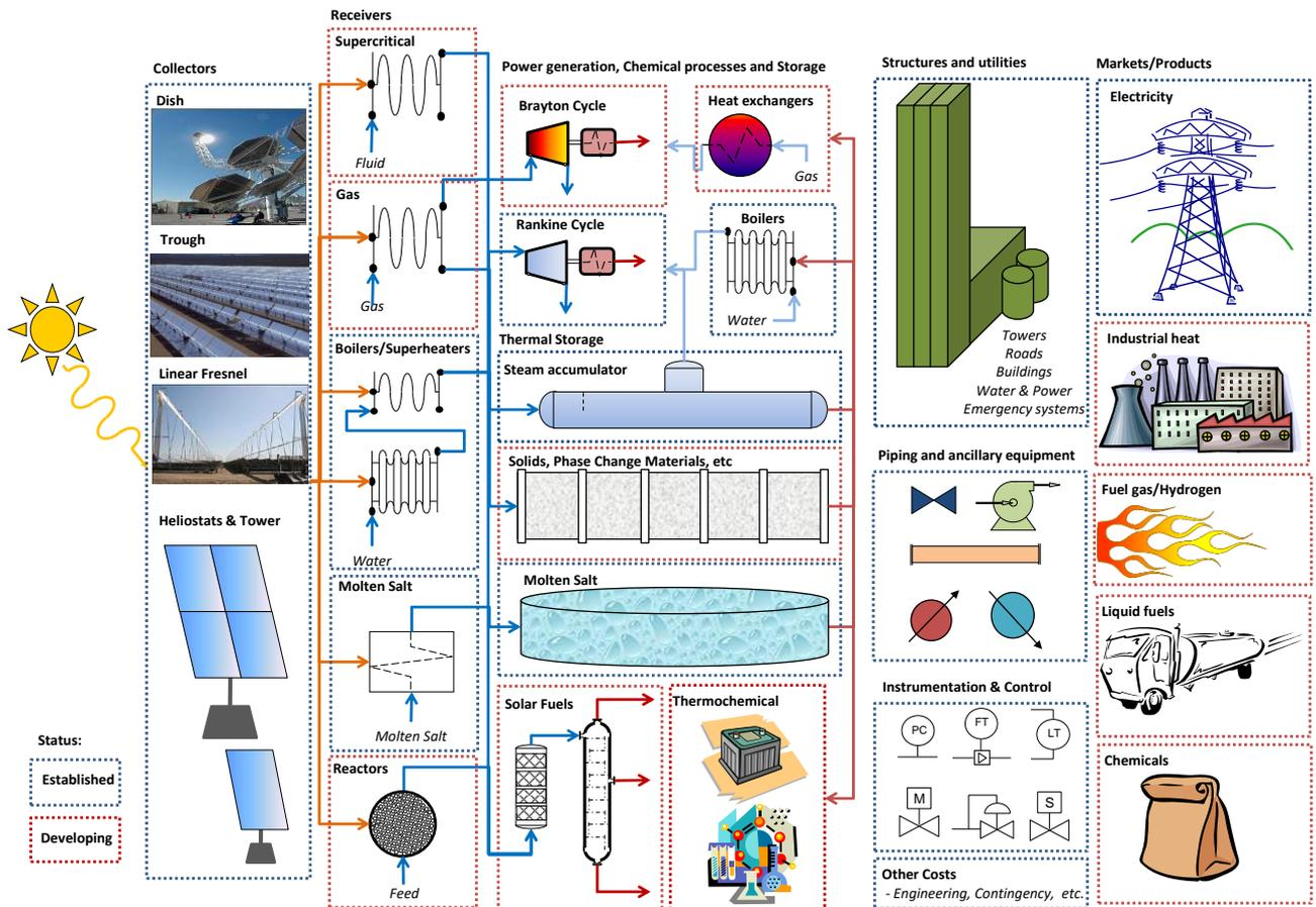
Figure 3.1: Established and Developing Solar Thermal Technologies and Market Applications
