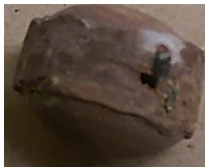
Figure 4.13 Geopolymer capsule showing leakage after 10 cycles
