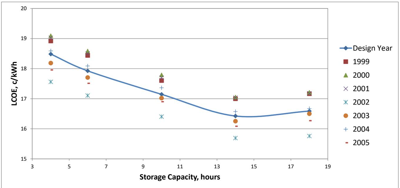
**Figure 4.3 - Variation in LCOE for varying plant sizes and storage capacities at Mildura for individual years of operation using historical solar data**
