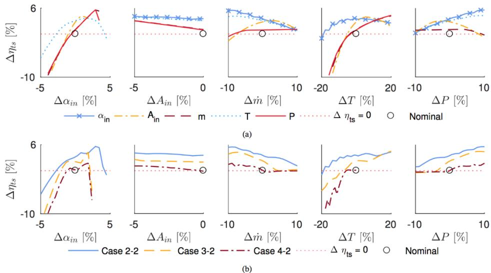
**Figure 4.28 Two-Way off-design optimisation showing a) correcting variable and corresponding maximum efficiency for Case 2-2 and b) composite efficiency for cases with different specific powers (Cases 2-2 and 3-2, CO2) and different curves fluids (Case 4-2, SF6)**
