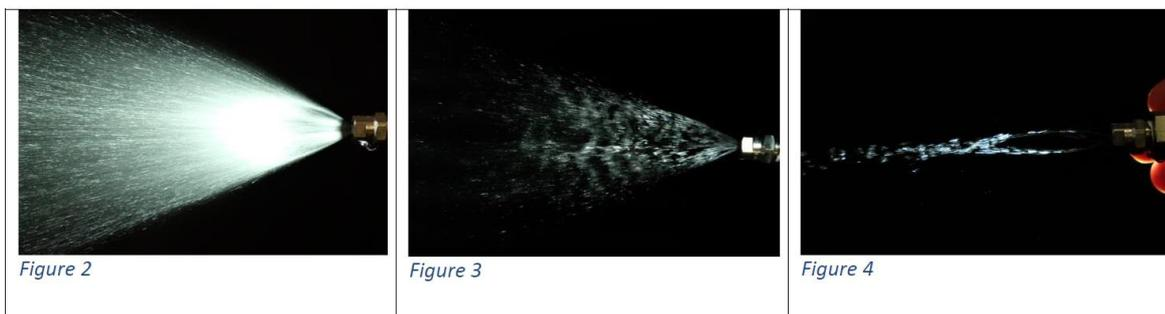
Figure 4.33B High-speed photography (Figure 2-4 ) of spray cleaning of mirror
