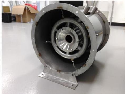
**Figure 4.43 Picture of the thermochemical reactor constructed at ANU for carbonate looping thermochemical energy storage**
