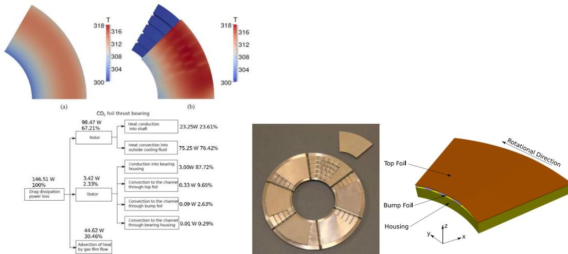
Figure 4.22: Results from a coupled fluid-structural-thermal simulation of a foil bearing operating with sCO<sub>2</sub>. Comparison to air bearings has highlighted a different distribution of heat loads, requiring a new approach to cooling. (Publication [3,5])
