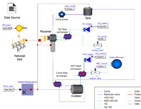
**Figure 4.52 Hydrogen production plant based on CeO<sub>2</sub> thermochemical redox cycle**
