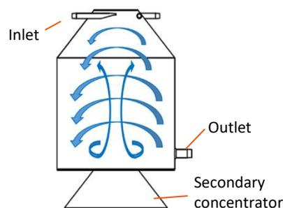
Figure 4.2. Simplified representation of the 3D flow-field within the SEVR
