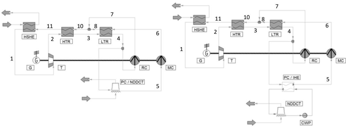
Figure 4.16: System models used for comparison of direct and in-direct cooled sCO<sub>2</sub> cycle.
