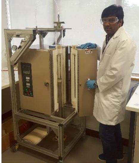
**Figure 4.41 Atmosphere controlled corrosion and high temperature density measurement rig at ANU**
