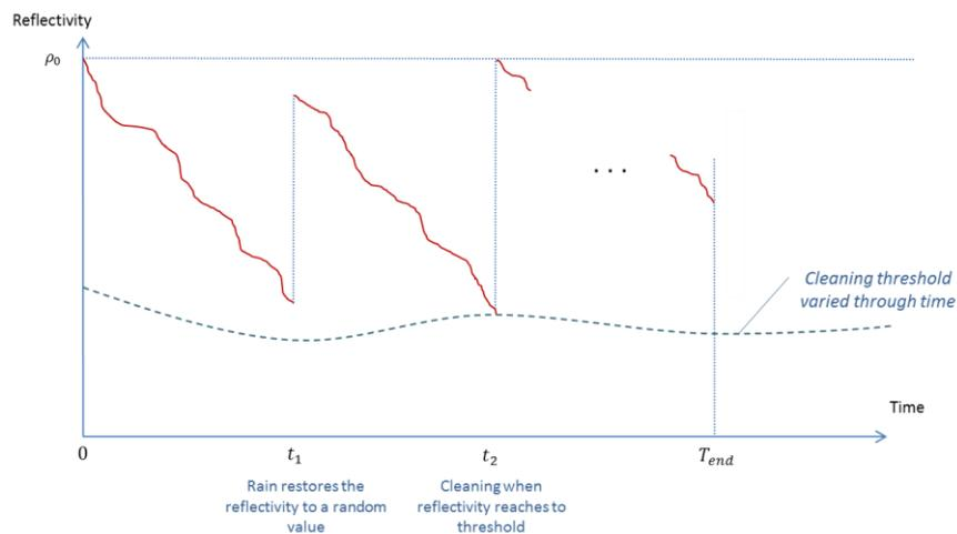
**Figure 4.33 Model concept of CBC methodology with reflectivity degradation and cleaning threshold**
