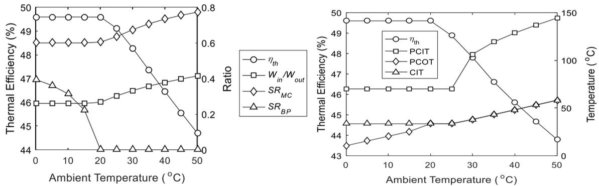
**Figure 4.19: Effects of ambient conditions on cycle performance for (a) direct and (b) in-direct cooled sCO<sub>2</sub> cycles, corresponding to cycle configurations from Figure 1.**
