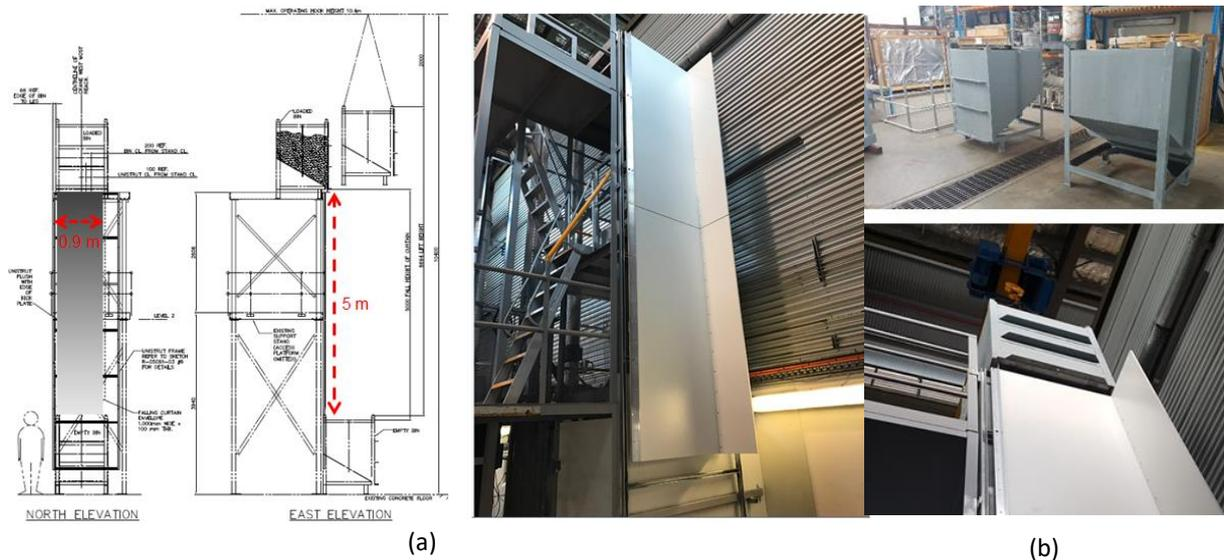
Figure 4.39. Cold-flow falling particle test rig at CSIRO showing (a) the tower and (b) the two particle hoppers used at top and bottom of the tower.
