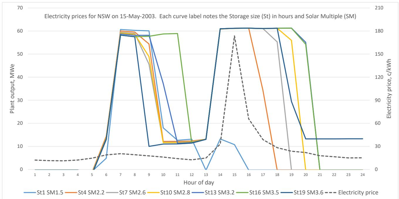
**Figure 4.5 - Example results of optimisation of plant design to match network electricity prices**
