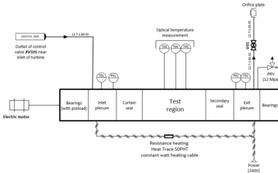
**Figure 4.47: Test arrangement for measuring the shaft heat transfer in supercritical CO<sub>2</sub> conditions. Using optical measurement techniques the temperature of the high speed shaft is monitored and the potential of different cooling arrangements can be evaluated.**
