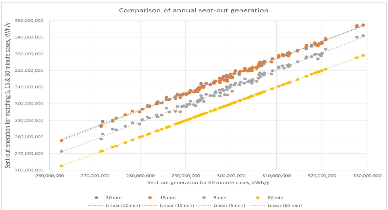
**Figure 4.4 - Influence of time resolution of solar data and annual variability on predicted plant output**
