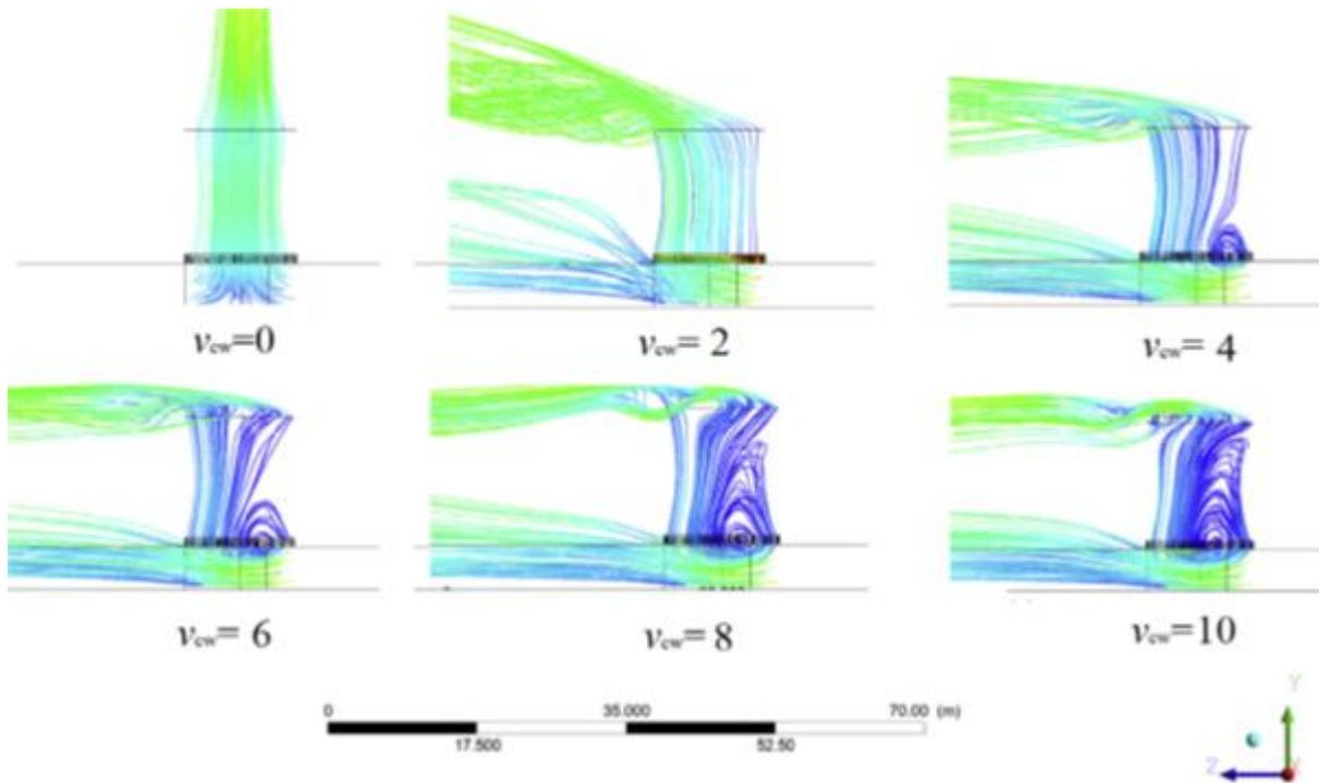
Figure 4.24 Modelling results of crosswind effect (with Gatton tower)
