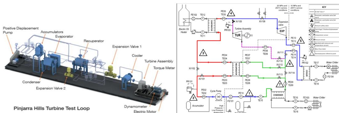
Figure 4.18: Pinjarra Hills High Pressure Test Loop. Now commissioned for sCO<sub>2</sub> operation. With upgraded pump capable of flows up to 0.25 kg/s and maximum temperature of near 250°C.
