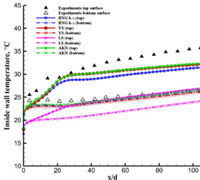
Figure 4.27 - Modelling results for sCO<sub>2</sub> heat exchanger with different models
