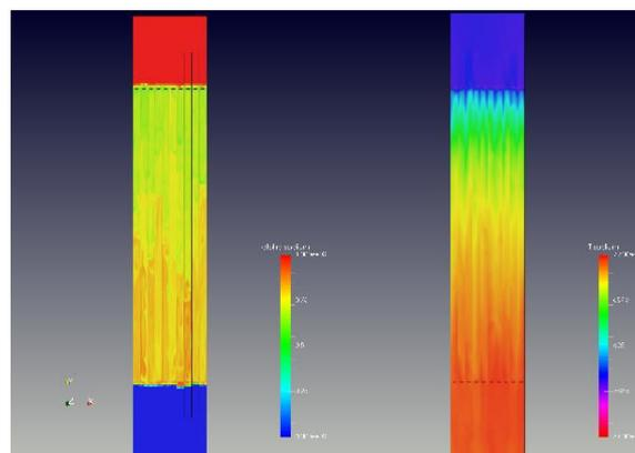
**Figure 4.42 Multichannel direct contact heat exchanger between sodium and molten salt. Figure shows the spatial distribution of sodium and the temperature distribution in the heat exchanger ( $\alpha_{\text{sodium}}$  is the phase fraction of sodium)**
