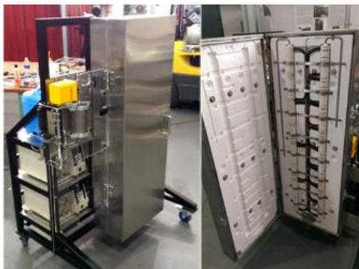
**Figure 4.50. Experimental rig for supercritical water gasification of biomass. Left: the complete system, mounted on wheels and ready for installation in a walk-in fume cupboard. Algae and water flow-rates are controlled by the two HPLC pumps at bottom left. Right: detail of the furnace section, where a U-shaped tube is fitted with electrical heating elements and with thermocouples to measure process temperature.**
