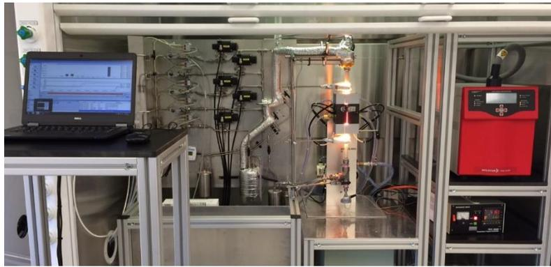
**Figure 4.51 Thermochemical materials testing facility. From left to right: Data acquisition PC, mass flow controllers with pneumatic safety valves, IR gold image furnace, and mass spectrometer (top right) and gold-IR furnace temperature controller (bottom right).**
