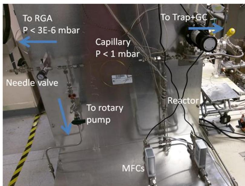
**Figure 4.53** Experimental setup for the flow-through continuous reactor for the advanced Sabatier process. A small quantity of metal-cluster based catalyst (10-50 mg) can be readily tested and the hydrocarbon product distribution determined rapidly via gas chromatography and mass spectrometry.
