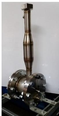
Figure 4.44 1-kW solar bubble receiver/reactor (UoA)
