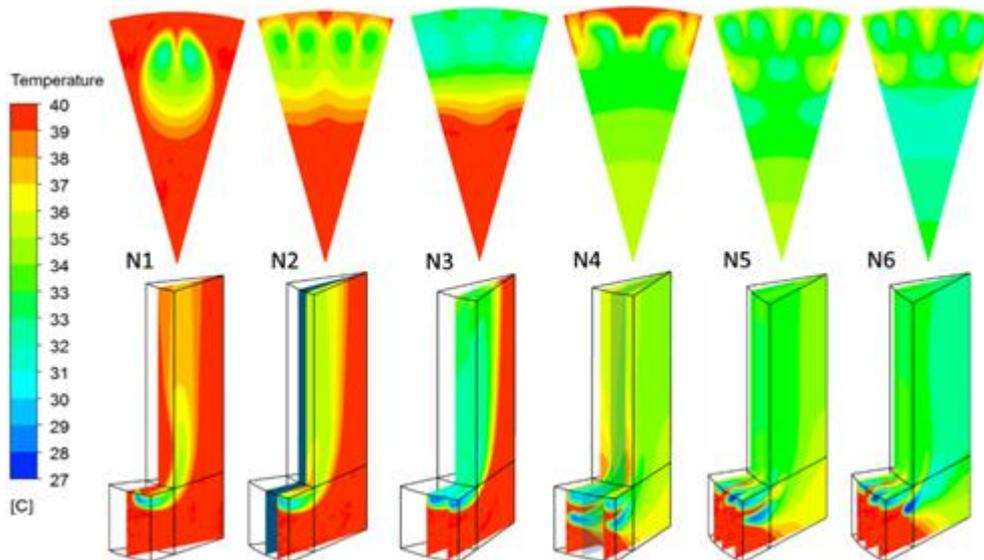
Figure 4.26 - Temperature profile in cooling tower with spray cooling
