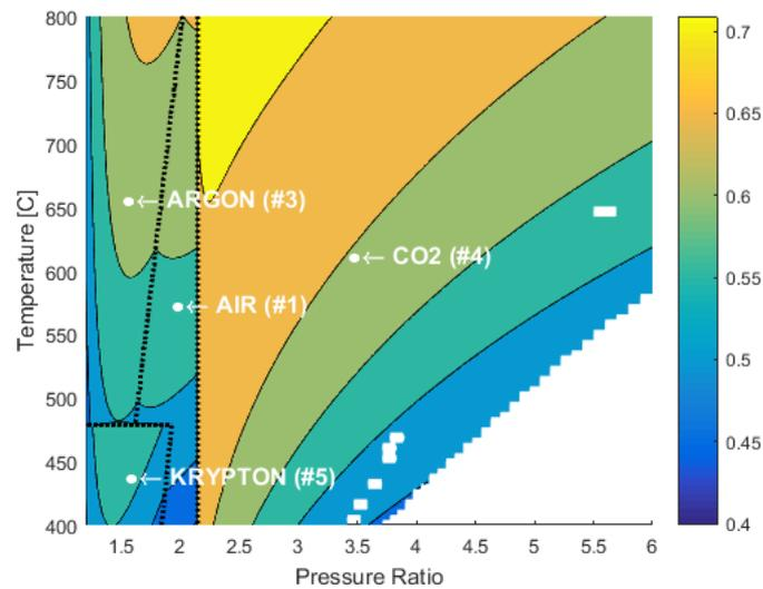
**Figure 4.29 - Parametric analysis of the effect that Pressure Ratio and Turbine Inlet Temperature has on fluid selection for the Recompression Brayton cycle. The chart shows that, for the given assumptions, for any pressure ratio above 2.1 CO2 results in optimal system efficiency.**
