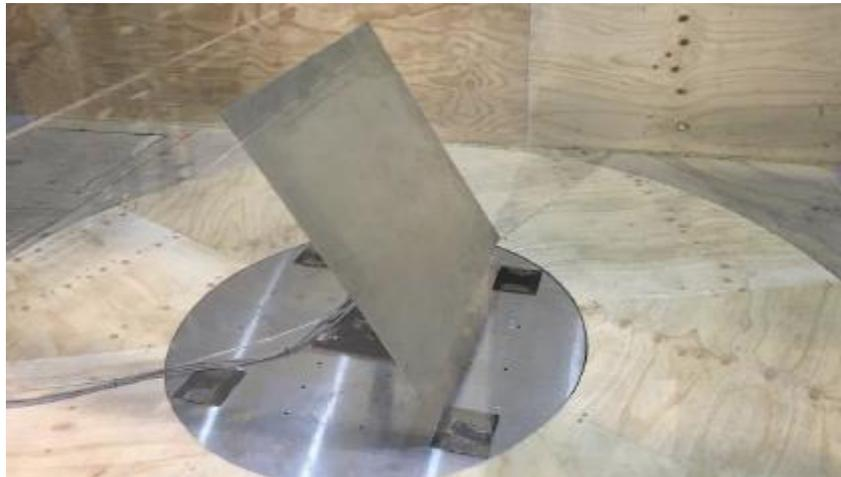
Figure 4.36 Heliostat scale model in Thebarton wind tunnel at the University of Adelaide
