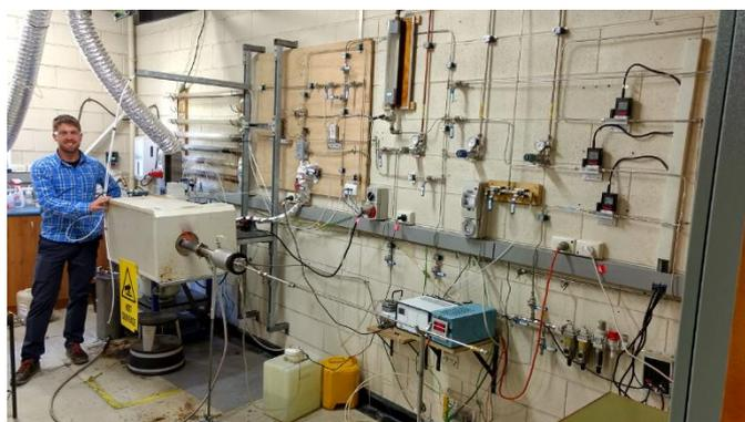
Figure 4.49 Experimental setup to simulate various SDFB environments to understand the mechanisms of agglomeration between the selected feedstock and bed material.
