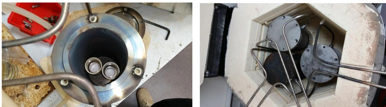
**Figure 4.15 Nitrogen atmosphere chamber with samples (left) and chambers placed in furnace (right).**
