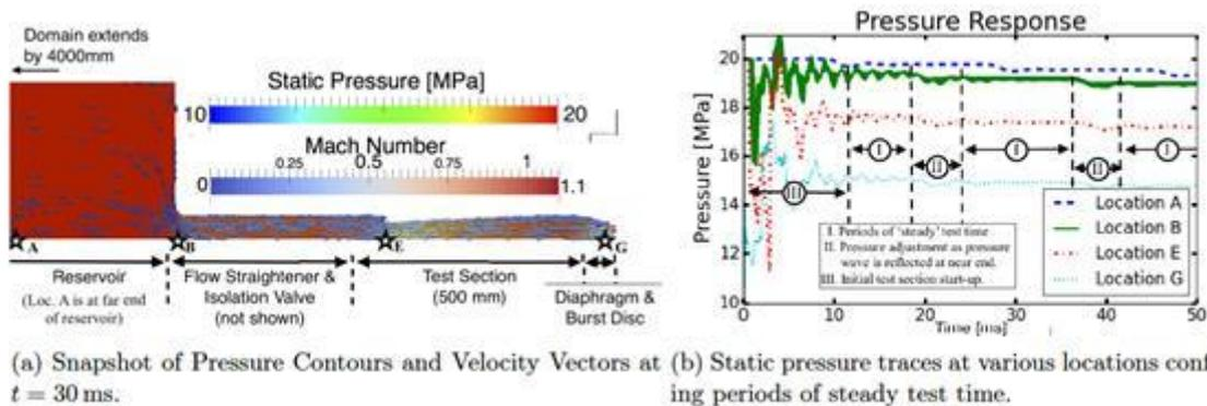
Figure 4.48: Test facility to create short duration high flow rate  $s\text{CO}_2$  conditions to investigate fundamental aerodynamics in supercritical  $\text{CO}_2$  flows.
