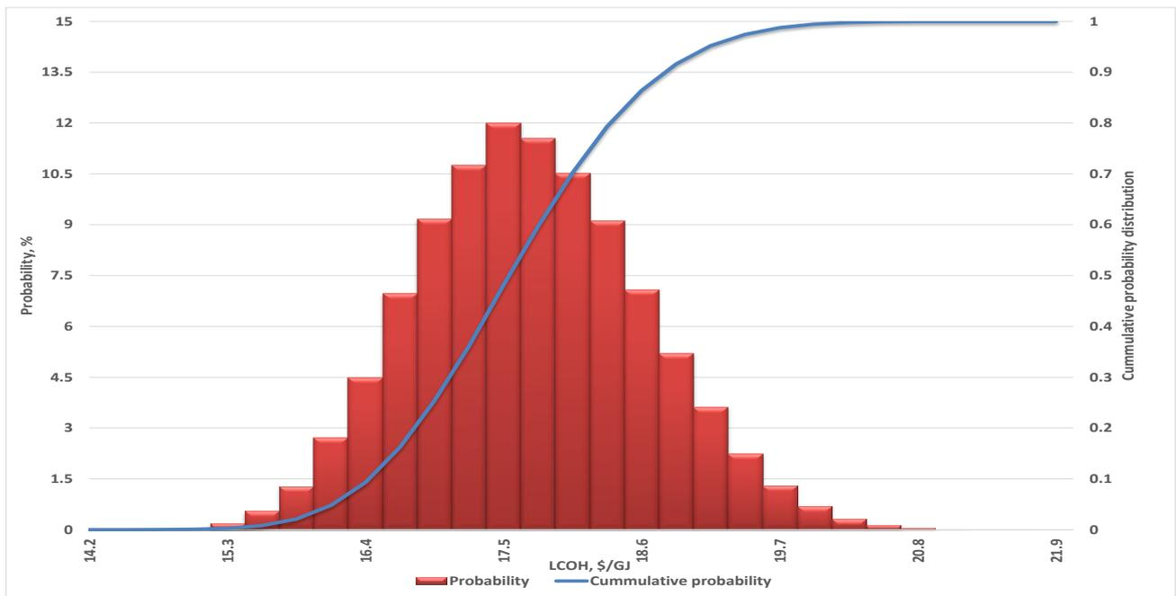
**Figure 4.6 - Probability distribution for the cost of high capacity factor industrial heat provision at 250MW<sub>t</sub> scale in Kalgoorlie**
