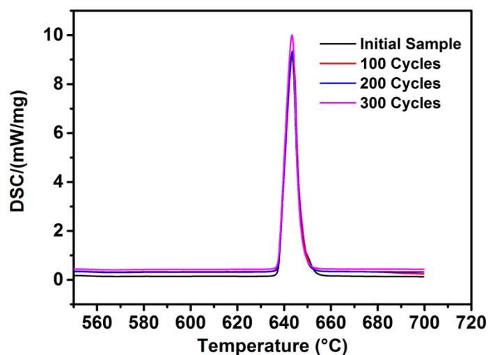
**Figure 4.14 Comparison of initial sample with 100, 200 and 300 cycles of eutectic Na<sub>2</sub>CO<sub>3</sub>-NaCl in a CO<sub>2</sub> atmosphere.**
