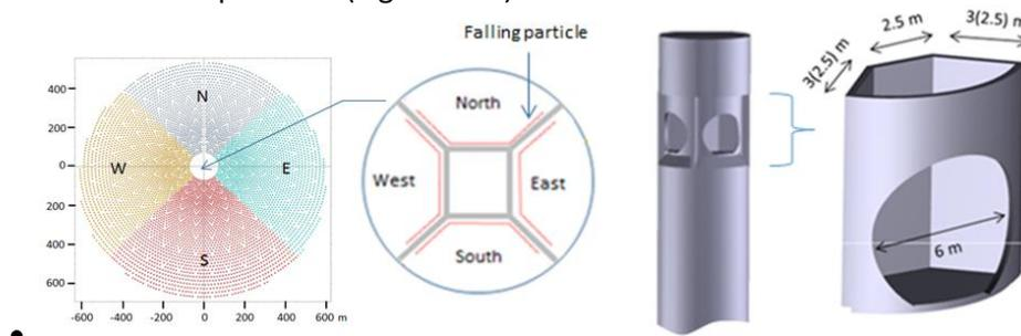
**Figure 4.3. Concept geometry of a receiver employing 4 cavities compatible with the ASTRI reference field optimised for a system in Alice Springs, Australia, (assumed heliostat size: 6.1 m x 6.1 m, number of heliostats: 6,177, tower height: 92 m).**
