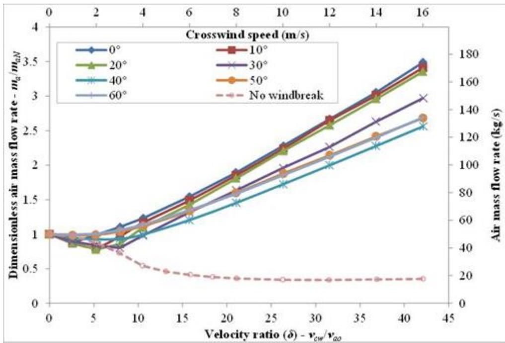
Figure 4.25 - Modelling shows windbreak wall significantly improving cooling tower performance
