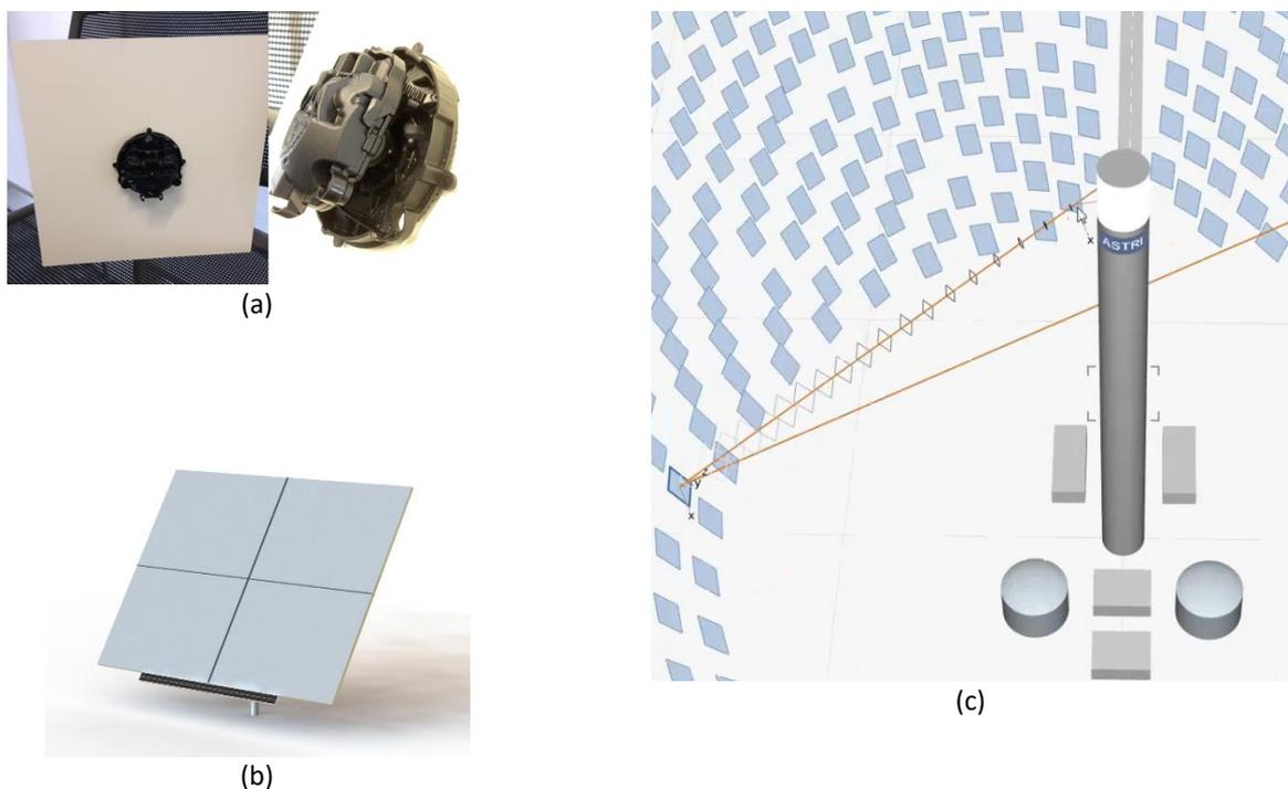
**Figure 4.7. (a) Mini-facet concept, with the automotive actuation device (b) the 30m<sup>2</sup> sandwich panel heliostat concept and (c) a snapshot of analysis in HELIOSTAT STUDIO.**
