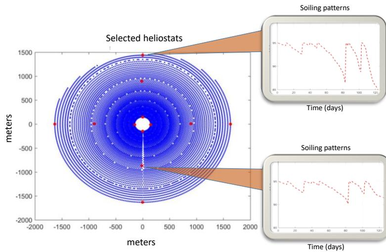
**Figure 4.37. Time-varying soiling degradation across the solar field**
