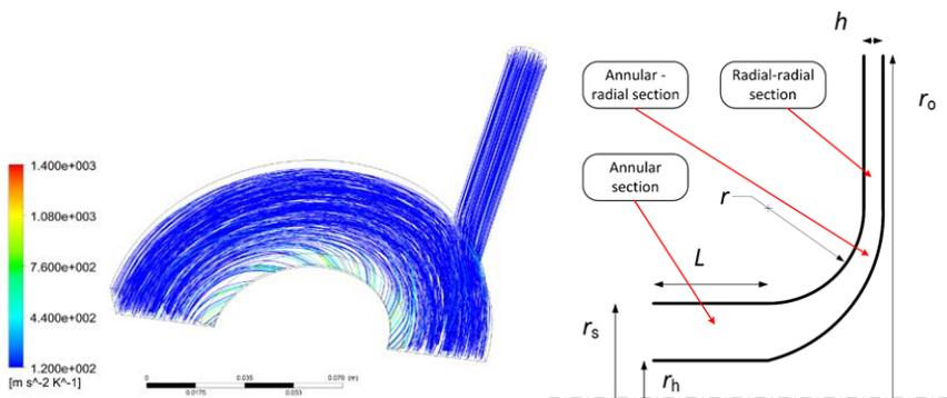
**Figure 4.20: Simulation results from an optimised inlet plenum and set-up of a design optimisation of a space constraint diffuser. (Publication [4,6])**
