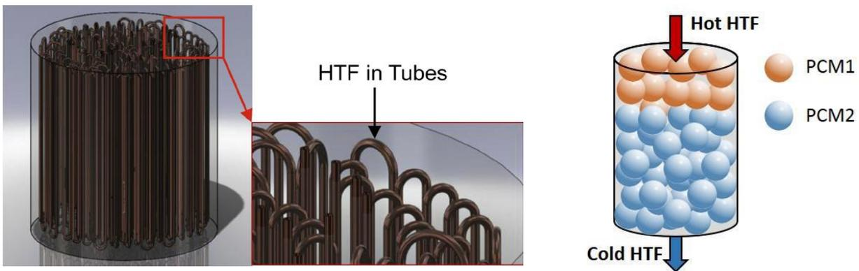
Figure 4.12. Schematic of coil-in-tank and packed bed system (with two different PCMs)
