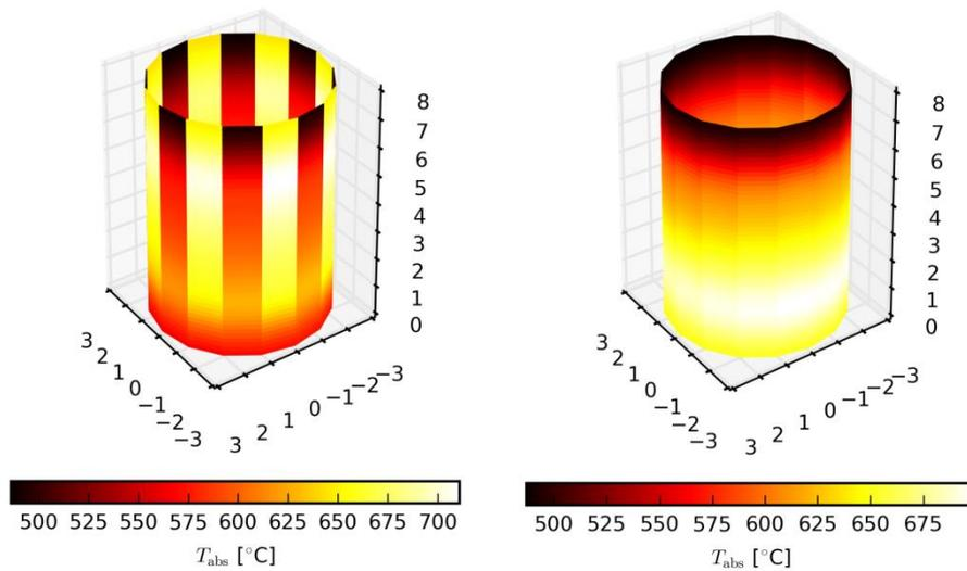
Figure 4.1. Absorber temperature distributions for a sodium receiver with 8 flow-paths, going down then up (left), and 16 flow-paths going down (right).
