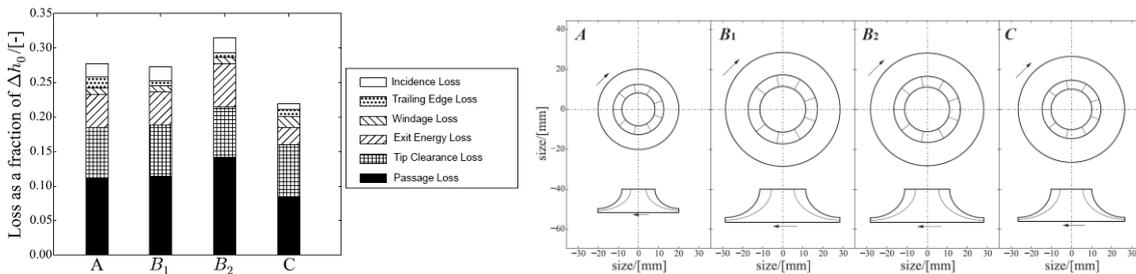
Figure 4.17: Results from a 0-D design space analysis for sCO<sub>2</sub> turbine rotors in the 100-200kW range. Trends between turbine style and loss contributors were identified from (Publication [2] ).
