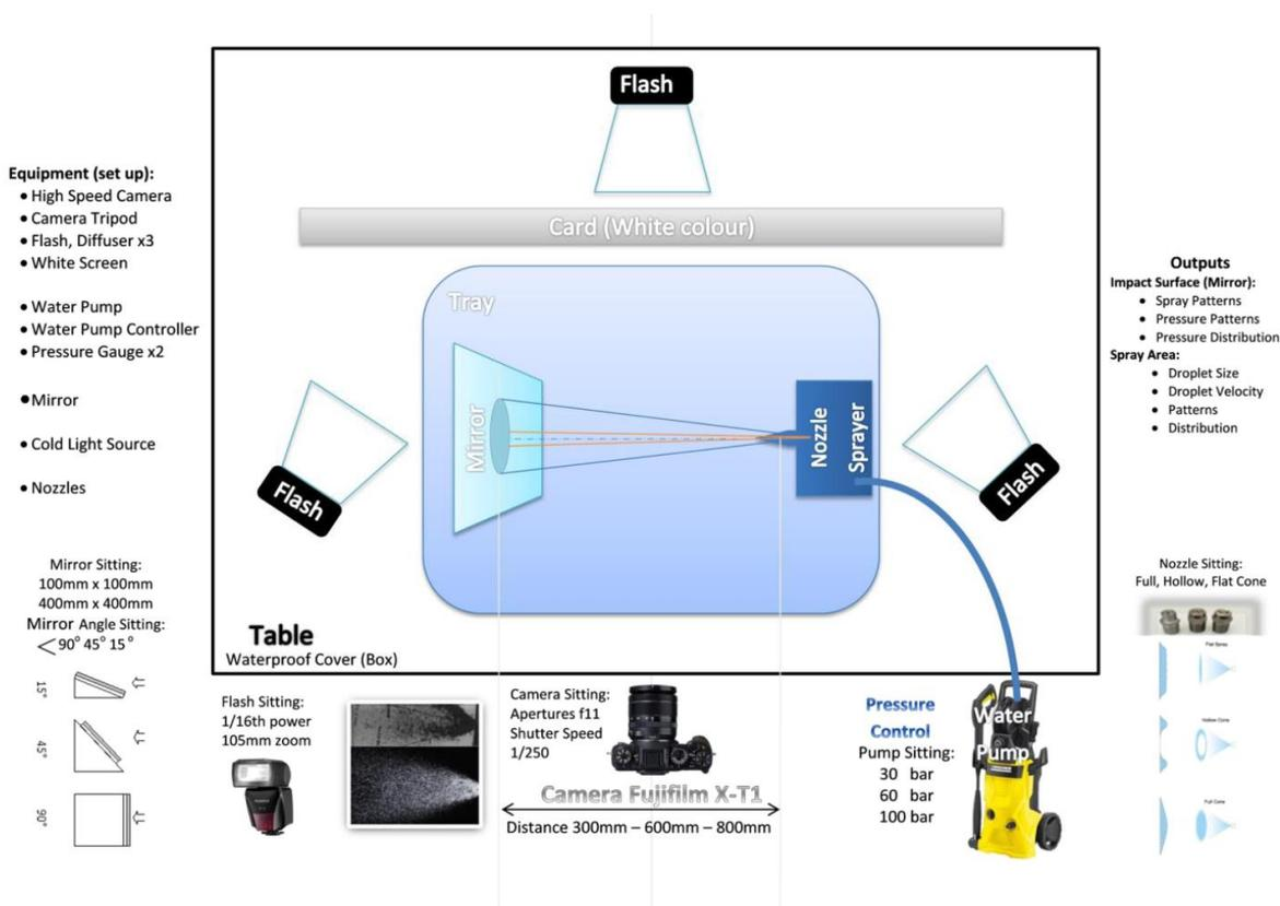
Figure 4.33A Set-up for mirror spray cleaning using high-speed camera to visualise spray.
