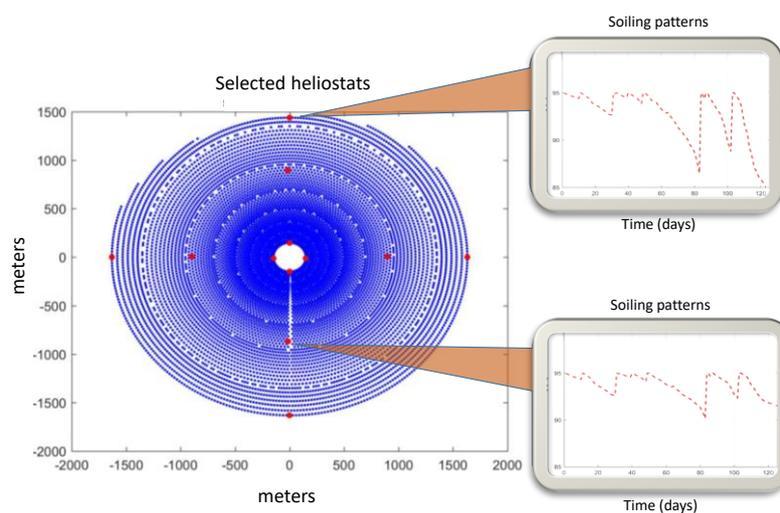
**Figure 4.30 - Time-varying soiling degradation across the solar field**
