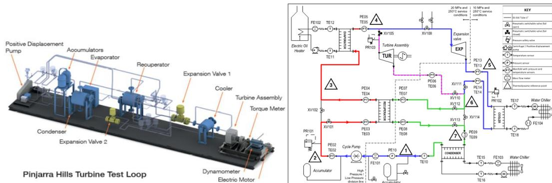
Figure 4.45: Pinjarra Hills High Pressure Test Loop. Now commissioned for sCO<sub>2</sub> operation. With upgraded pump capable of flows up to 0.25 kg/s and maximum temperature of near 250°C.
