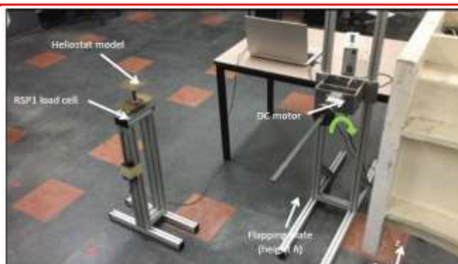
A 'flapping plate' vortex generator for testing some large-scale turbulence structures that can be expected in the upstream wind within heliostat fields
