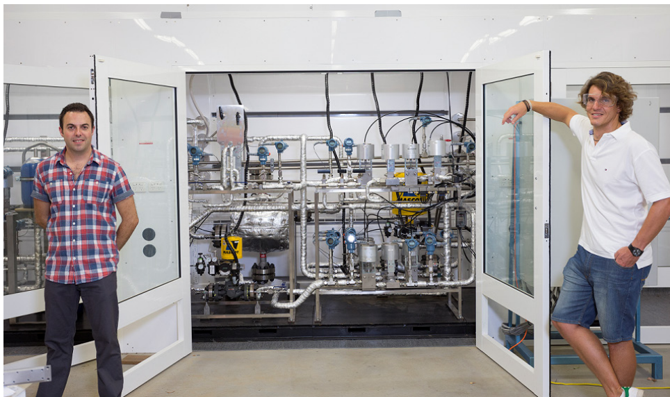
The University of Queensland High Pressure Turbine Test Rig with Andrew Rowlands (L) and Carlos Ventura (R)
