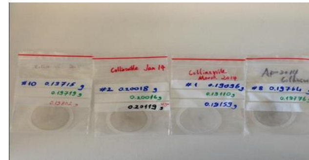
Filters collected at Collinsville with different dust concentration
