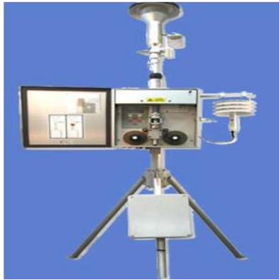
Airborne dust monitor
