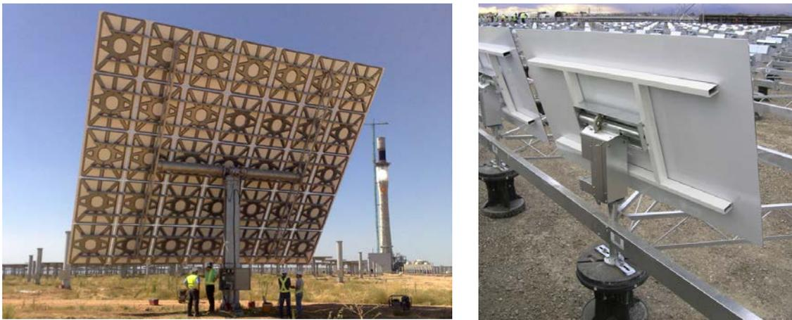
Figure 4. 115.7 m<sup>2</sup> Sener heliostat (left) and 1.14 m<sup>2</sup> eSolar heliostat (right) [13, 22].
