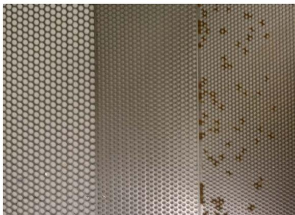
**Figure 29. Fence models used for porosity study (from left to right: 58%, 46%, 40% open area) [37]**
