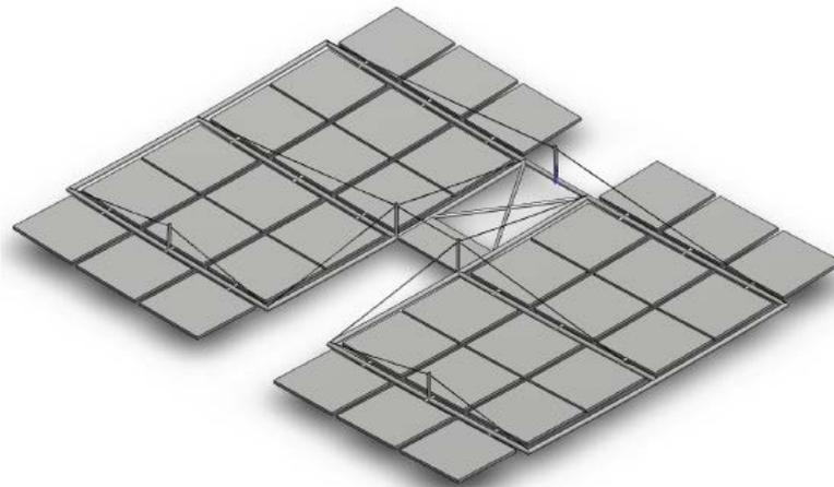
**Figure 10. JPL/L'Garde heliostat concept [26]**
