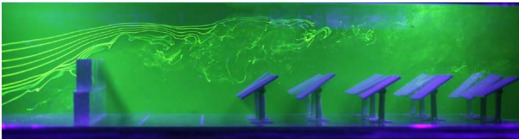
**Figure 28. Visualization of the flow over the heliostat field with a solid barrier placed in front [37]**
