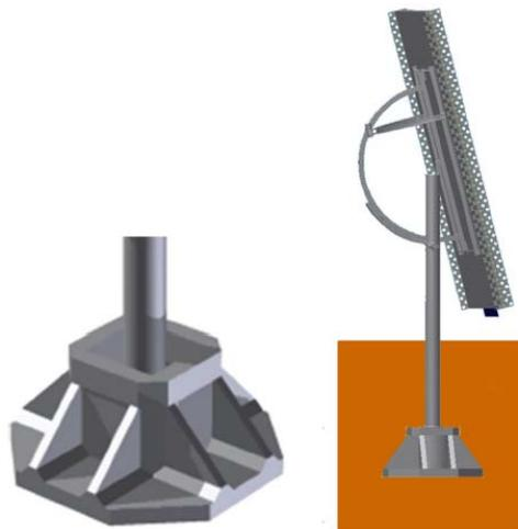
**Figure 72. Pre-fabricated concrete ground-anchor foundation**
