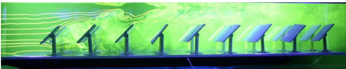
**Figure 31. Visualization of the flow over a heliostat field**
