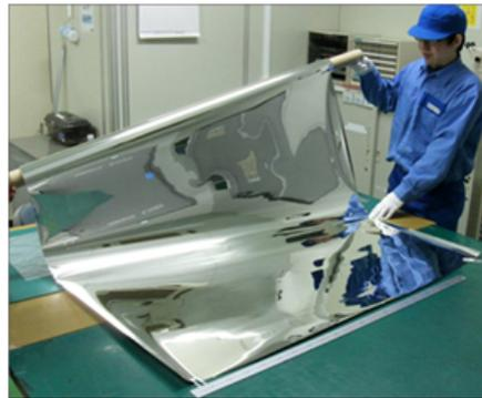
**Figure 40. Konica Minolta's new 1.3 m wide reflective film [132].**
