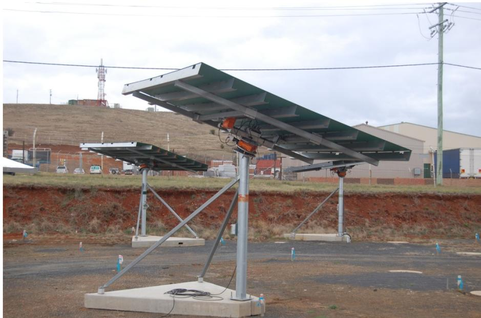
**Figure 14. Heliosystem's passive adjustment toroidal heliostat (PATH) [photo: Joe Coventry]**
