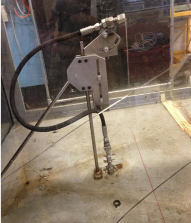
Set-up of spray nozzles.
